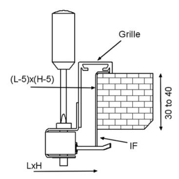
Concealed screw fastening is possible when the grille is installed with an installation frame (IF).
