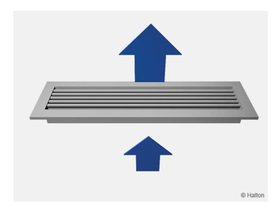
Supply air is supplied without deflection through the horizontal vanes into the space. Supply air mixes with room air in front of the grille.
