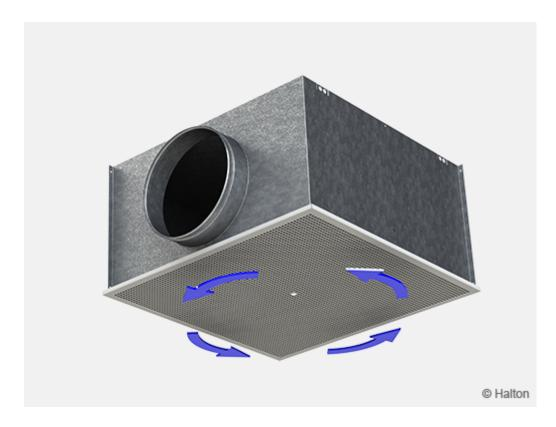
Horizontal radial swirl jet is supplied into the space through the profiled spiral blades of the diffuser. Supply air jet velocity is efficiently reduced due to the high mixing effect.
