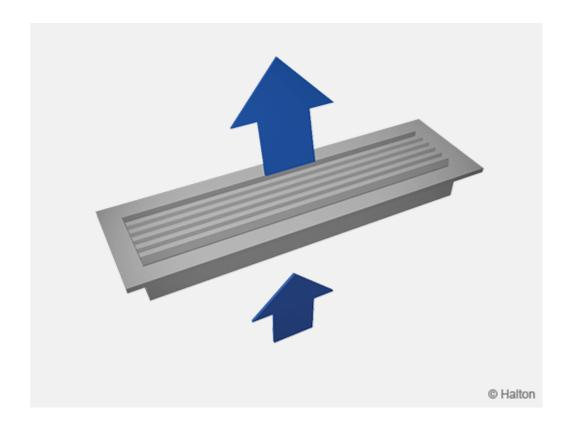
Supply air is supplied with a  $15^\circ$  angle deflection through the horisontal vanes into the space. Supply air mixes with room air in front of the grille.
