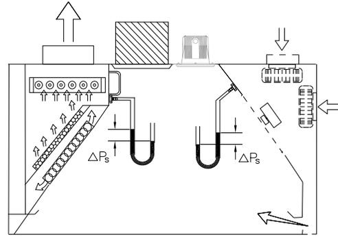
Exhaust air flow vs. pressure differential
