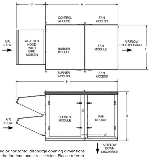
**Note:** Downward or horizontal discharge opening dimensions will depend on the fan type and size selected. Please refer to the job-specific submittal drawings for these dimensions.
