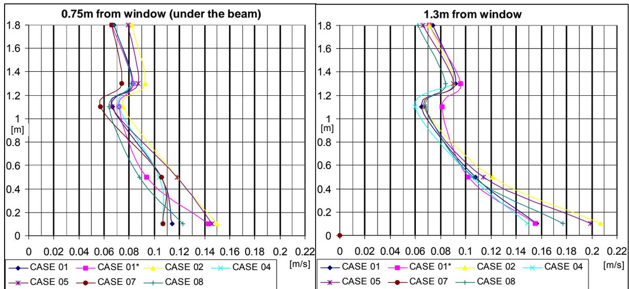
Figure 6. Velocity measurements at different heights from floor under the beam and at 1.3m distance from the window
