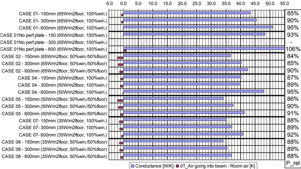
Figure 5. Conductance of the chilled beam and temperature difference between air going into passive beam and room air. Relative cooling capacities of the beam on the right side.
