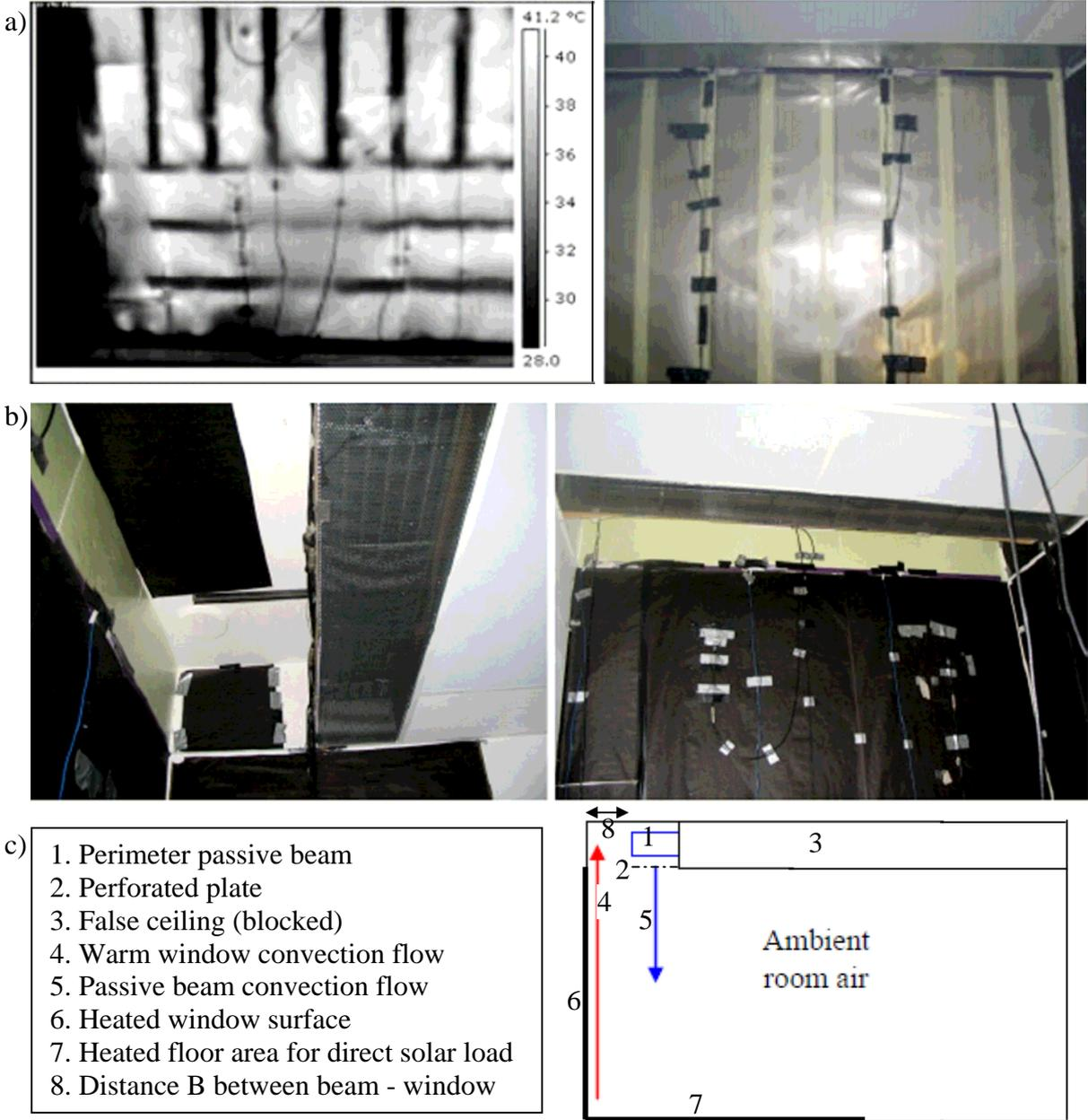
Figure 1. a) Arrangement of electric heated foil for solar load (infrared picture on left), b) installation of the perimeter passive beam and c) side view of installation with different components
