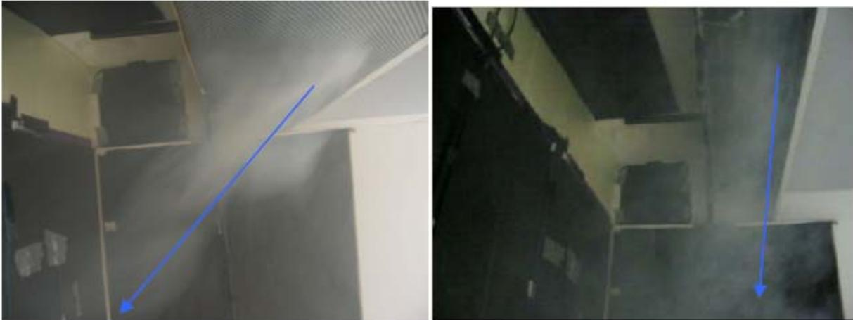
Figure 4. Smoke visualization of convection flow from passive beam. Measurement with perforated plate under the beam (left) and without perforated plate (right)
