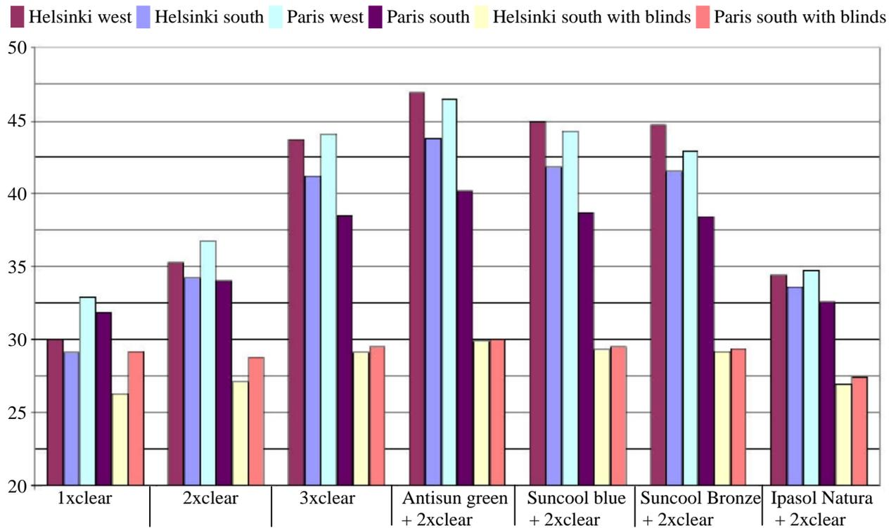
Figure 3. Window surface temperatures [deg C] during peak moment
