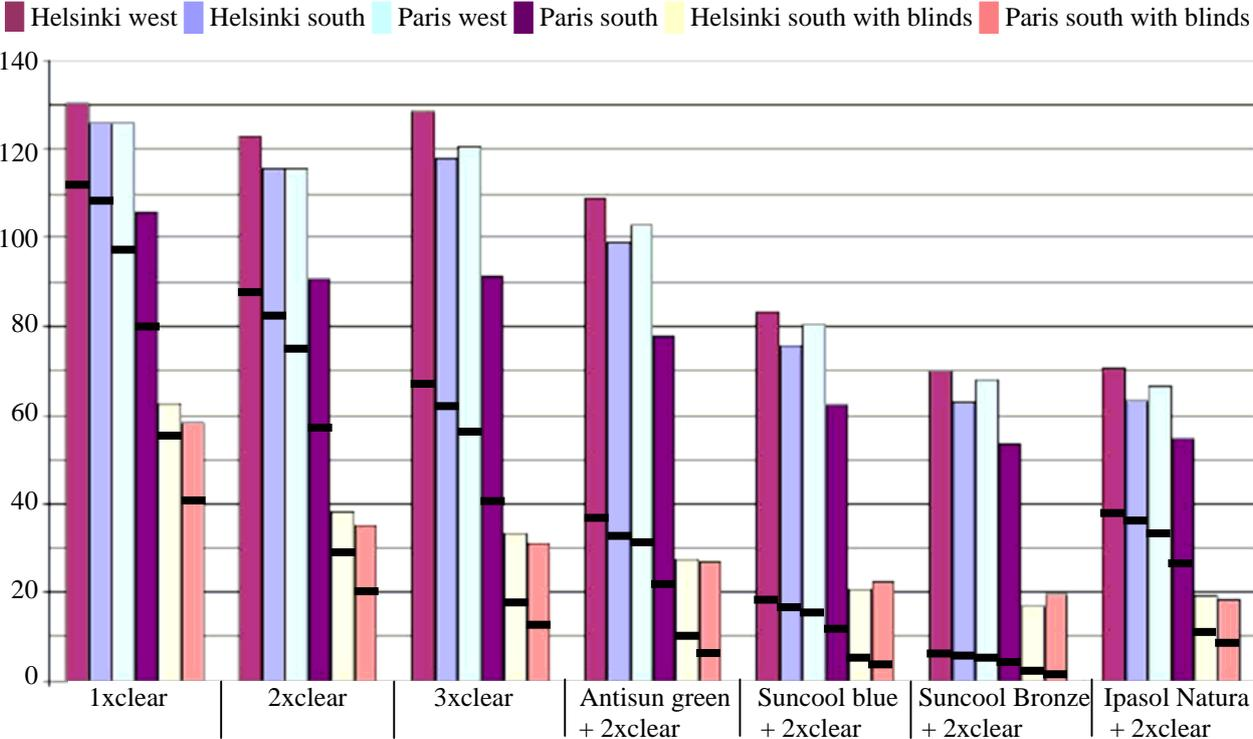
Figure 2. Total heat load [W/m<sup>2</sup><sub>floor</sub>] from the window with different window types. Direct and diffuse solar radiation heat load portion [W/m<sup>2</sup><sub>floor</sub>] below thick parting line
