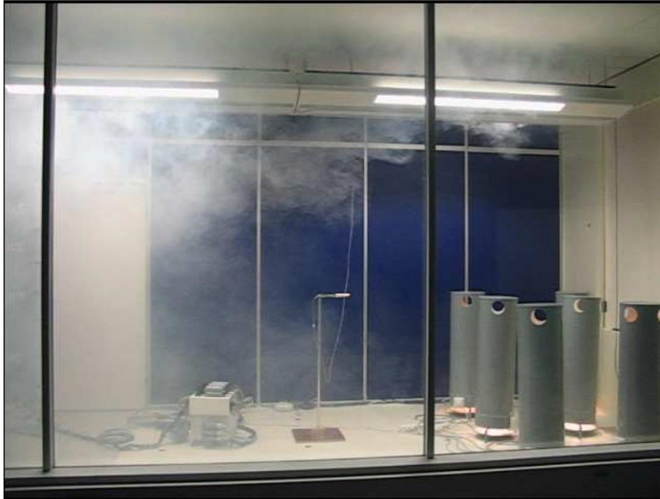
Figure 5. Smoke visualization when all heat sources are located closet to the window wall.
