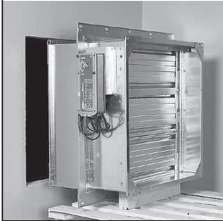
**6** The space between the wall and the fire damper is filled with non-combustible mineral wool with a density of min. 40 kg/m<sup>3</sup>.
