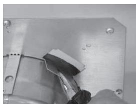
**8.** When the power is off, the electric actuator can be tested manually by means of a hexagonal spanner (included in the delivery).
