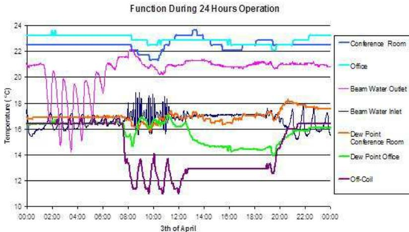
Fig. 4. The operation conditions in the ventilated beam system during one working day.
