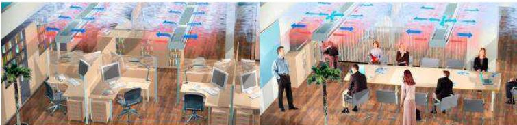
Fig. 3 Minimum office requirement is supplied through nozzles (left). In case of a high maximum airflow rate, air quality controller is introduced (right).
