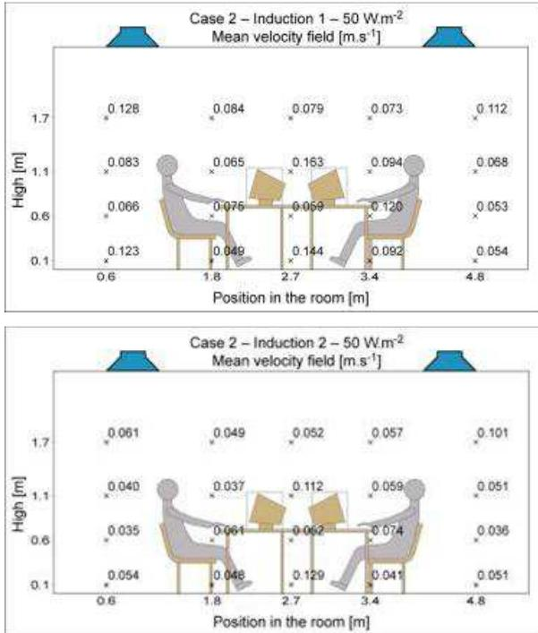
Fig. 2 Impact of induction ratio adjustment on air velocity in laboratory tests. Upper Image: Induction ratio adjustment off. Underneath image: Induction ratio adjustment on.
