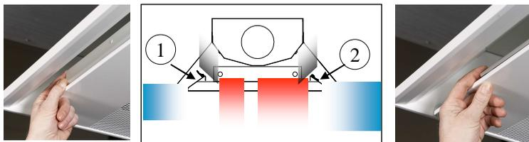
Fig. 1 Principle behind induction ratio adjustment: 1) induction ratio adjustment on and 2) induction ratio adjustment off.
