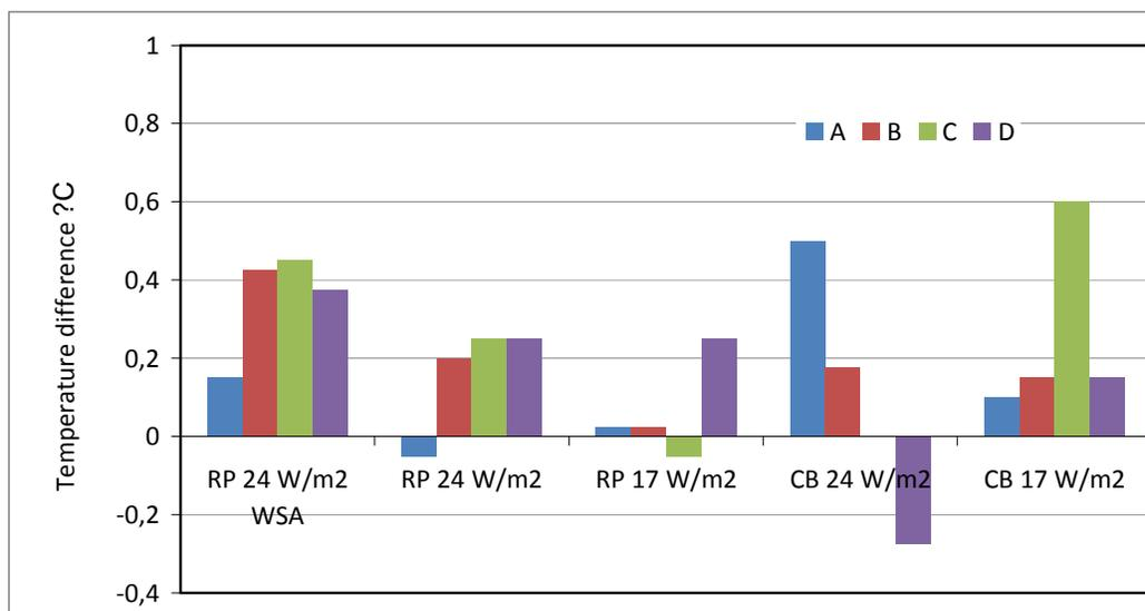
Figure 5. Difference between room air temperature and operative temperature measured at locations A, B, C, D at 1.1 m level above the floor in heating mode cases (WSA=without supply air).
