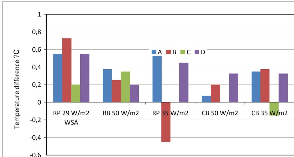
Figure 4. Difference between room air temperature and operative temperature measured at A, B, C, D at 1.1 m level above the floor in cooling mode cases. (WSA=without supply air)
