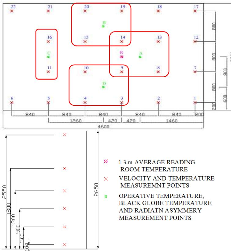
Figure 3. Measurement locations and heights in the room.
