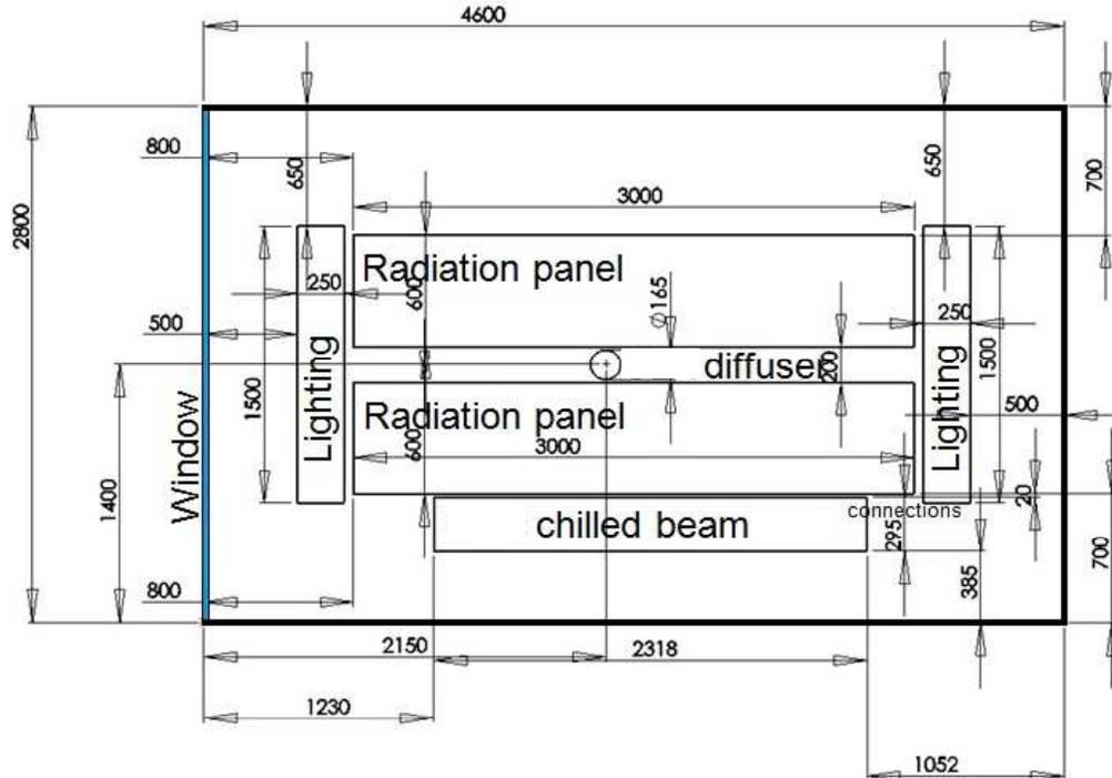
Figure 1. Set-up of the two systems studied.
