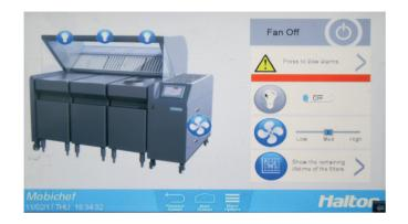
The user interface has been designed to manage advanced technologies by use of clear visuals which allows easy control of the main functions. The remaining life time of the filters are clearly displayed so that the maintenance operations can be easily planned.
