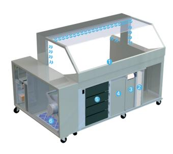
Halton Marine's MobiChef is equipped with the Capture Jet™ technology that "locks" the upper part and the side of the units by creating air curtain efficiently capturing smoke and odours released by the cooking process. The Capture Jets steer the smoke and odours to KSA multi-cyclone filters of the air recycling unit.
