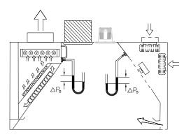
Exhaust air flow vs. pressure differential
