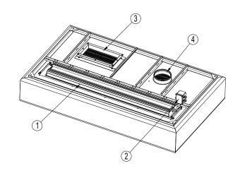
PARTS: 1 Lighting fixture, 2 Lighting fixture power supply junction box, 3 Eurovent-collar with flange, Lcollar available as an option, 4 Round duct connection, available as an option
