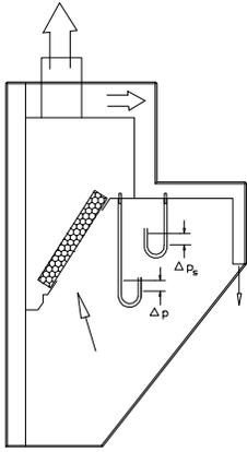
The capture jet and exhaust air flows are easily and accurately determined by measuring the pressure difference from the T.A.B.™ ports mounted in each plenum. Corresponding air flows can be read from the diagrams provided.
