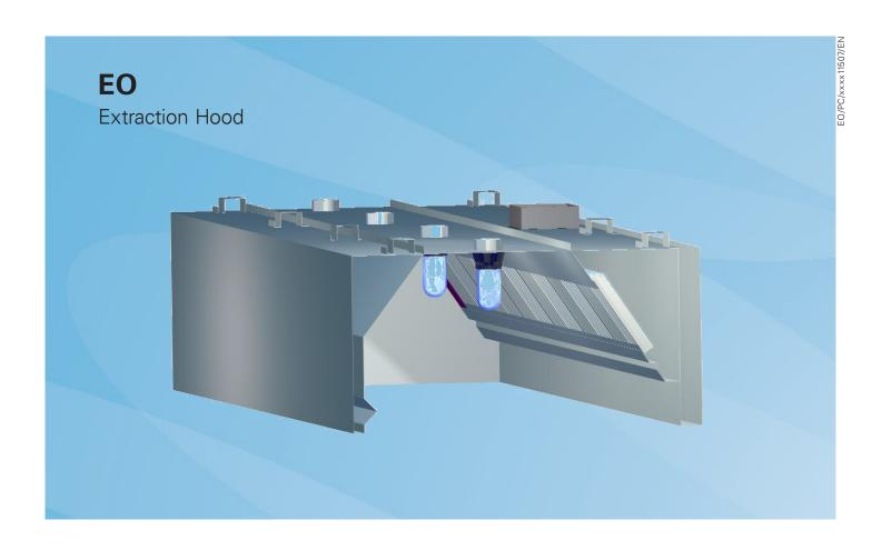
The EO hood is an extraction hood for exhaust of contaminated air released by cooking equipment with low heat loads. The hood is UL listed at 150 cfm per linear foot for light duty applications.
