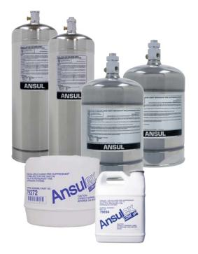
The tank is constructed of stainless steel. Tanks are available in two sizes: 5.7 | (1.5 gal) and 11.4 | (3 gal). The tanks have a working pressure of 7.6 bar, a test pressure of 22.8 bar, and a minimum burst pressure of 41.4 bar.
