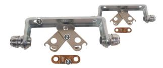
The detectors build up a detection chain along the exhaust plenum of the kitchen ventilation systems. They consist of three basic components: the bracket (1), the linkage (2) and the fusible link (3).
