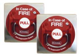
The remote manual pull station permits quick, sure manual actuation of the system by anyone regardless of fire fighting experience. It is equipped with a break rod indicating manual system operation. The remote manual pull station should be mounted at a point of egress and positioned at a height determined by the authority having jurisdiction.
