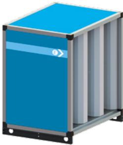
Built-in attenuators are available for PolluStop, Aerolys and Extenso with the option of Melinex lining for polluted airstreams. Intended for the reduction of in-duct noise transmission. Standard construction is 100mm Airways & 200mm Splitters, with 900mm, 1200mm and 1500mm length options. For specific noise requirements, consider seeking professional acoustic advice.
