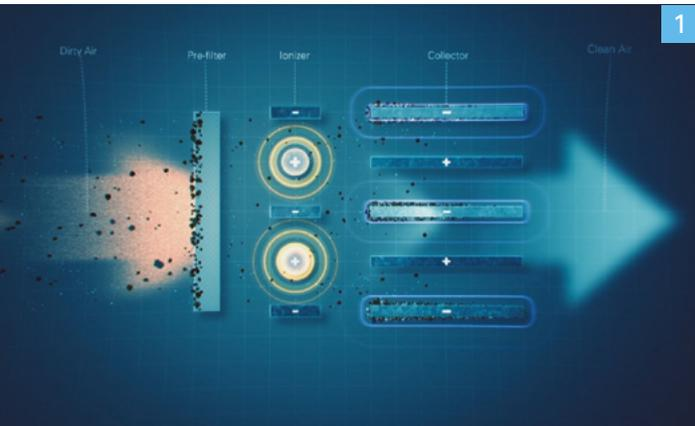
1 - Halton's ESP removes most of the unwanted moisture from the airstream along with much of the particulate matter generated by the cooking process.
