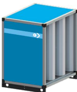
Built-in attenuators are available for PolluStop, Aerolys and Extensio with the option of Melinex lining for polluted airstreams. Intended for the reduction of in-duct noise transmission. Standard construction is 100mm Airways & 200mm Splitters, with 900mm, 1200mm and 1500mm length options. For specific noise requirements, consider seeking professional acoustic advice.
