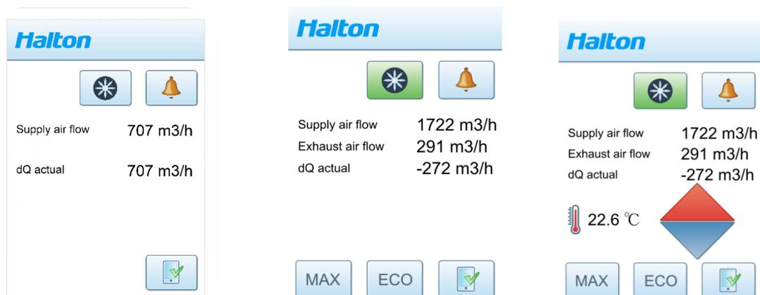
Fig. Halton HTP end-user views for VLR Room Airflow Control
