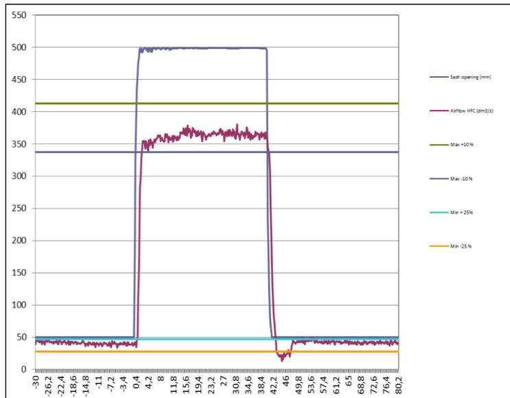
Figure: Double Sensor Control, system stability and reaction time
