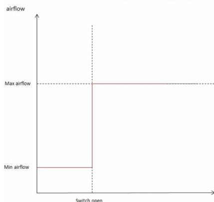
Figure: Dual position airflow control
