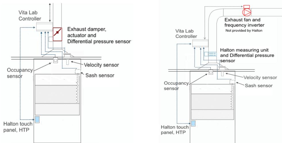
Figure: Double Sensor Control with centralised and single exhaust fan ventilation
