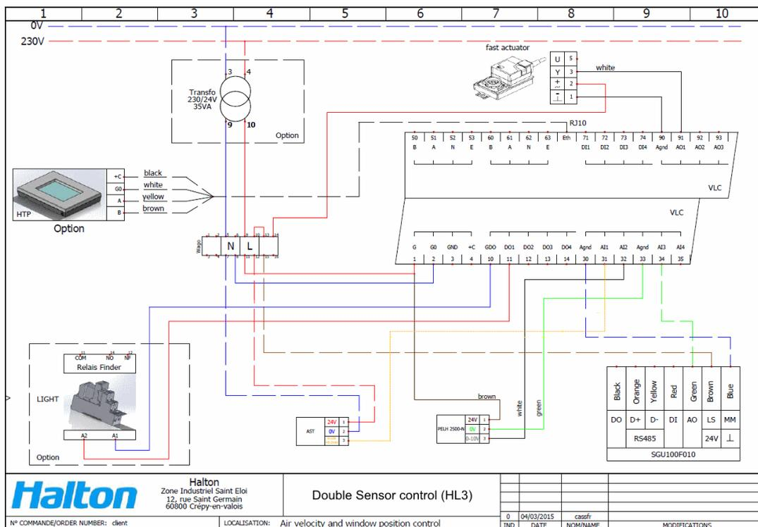
Figure: Wiring diagram for Double Sensor Control, centralised exhaust ventilation design
