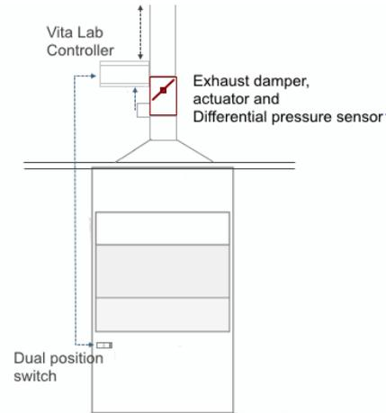
Figure: Dual Position Control, centralised exhaust ventilation
