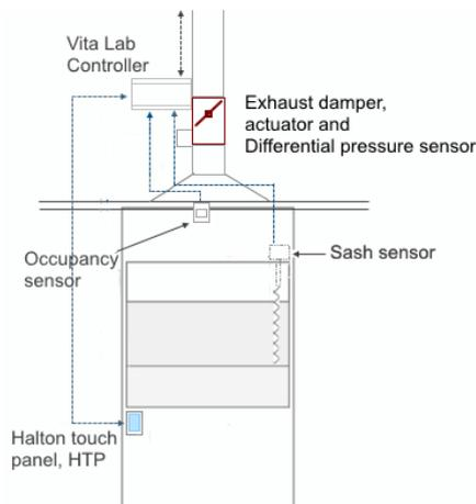
Figure: Sash Position Control, centralised exhaust ventilation
