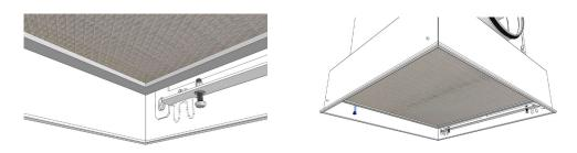
4. Ensure that the filter is centred and pressure measurement hose is visible on the side of the filter. Tighten the filter evenly, in crosswise sequence, with screws in the brackets until the screws bottom out.
