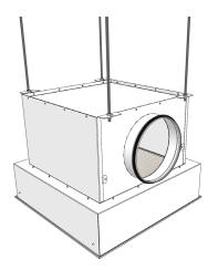
**NOTE:** Brackets can be bent 90° to support this method.
