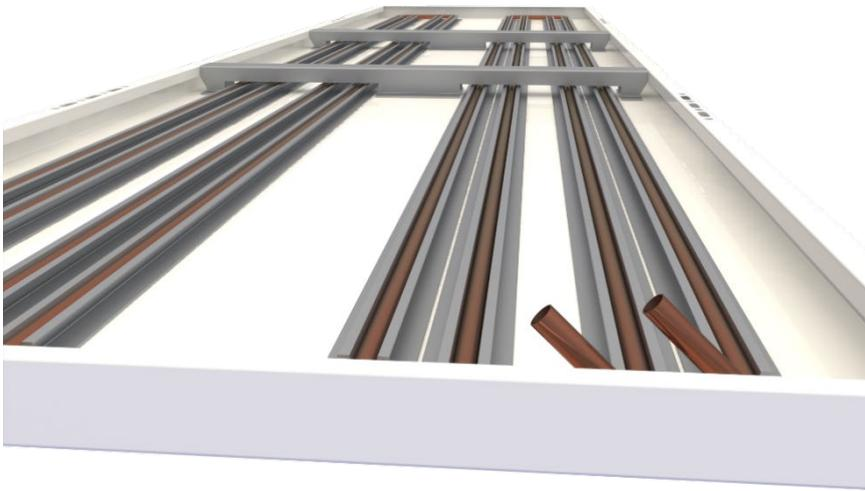
*Fig. 5. Connection pipes in two-loop panel (NL=2)*
