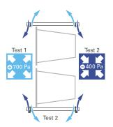
The air leakage in volume per unit of time [I/s m²], related to the external casing area. The test is carried out under a negative pressure of 400 Pa and a positive pressure of 700 Pa.
