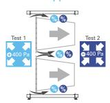
Air bypass around filter cells as a percentage of rated air volume flow.
