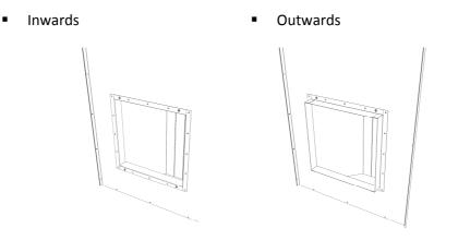
5. At this stage, the exhaust duct should be covered with a wall element. The wall element should have a hole for the grille. Check the hole dimensions from the table below.
