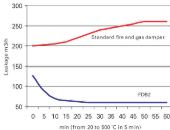
Graph 1. Leakage rate of Halton gastight fire damper in high heat.
