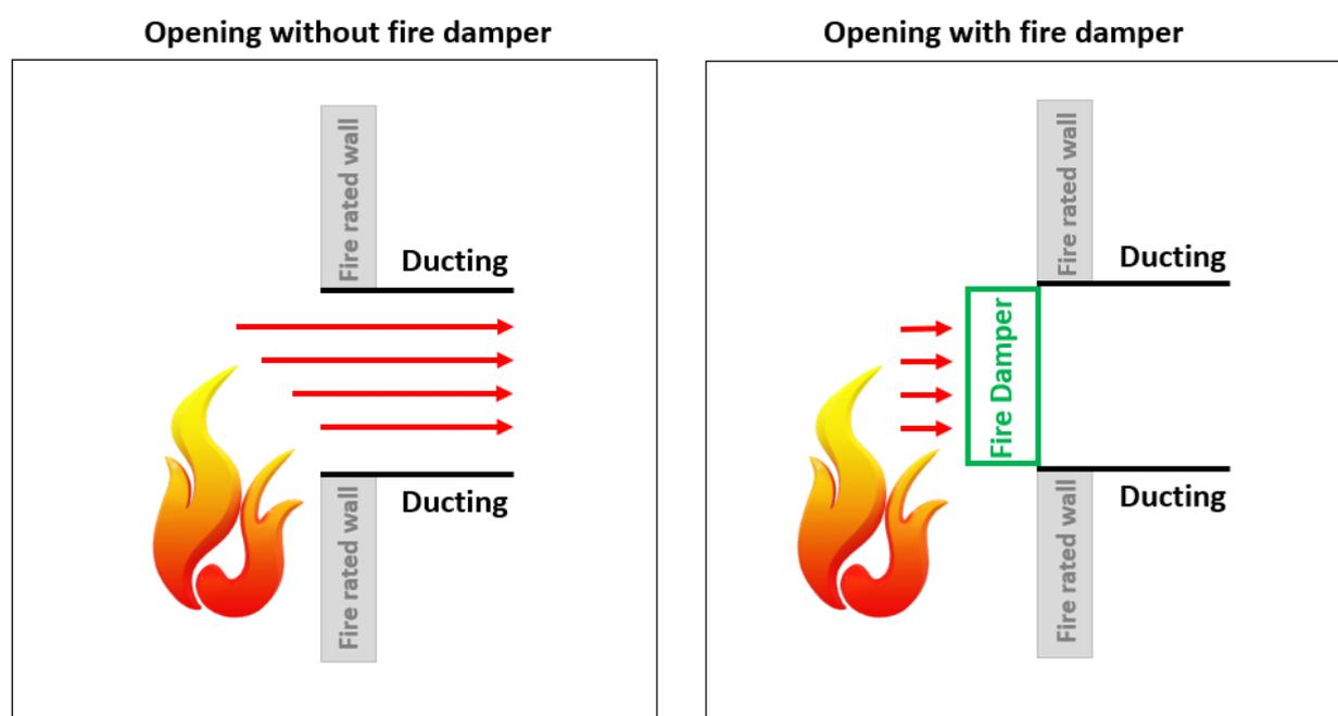
Picture 1. Fire Damper preventing the fire from spreading.
