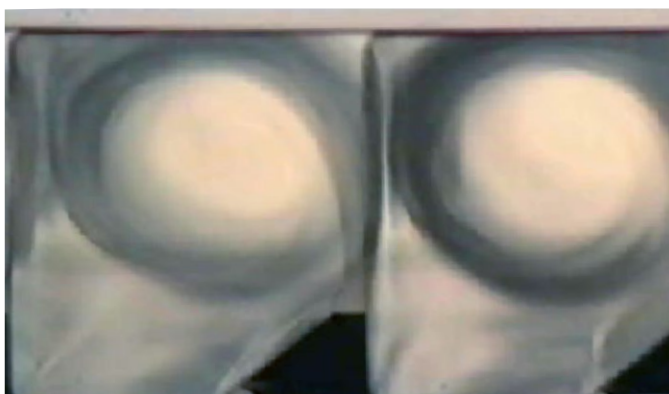
View on the cyclonic effect inside a KSA filter (Schlieren view)
