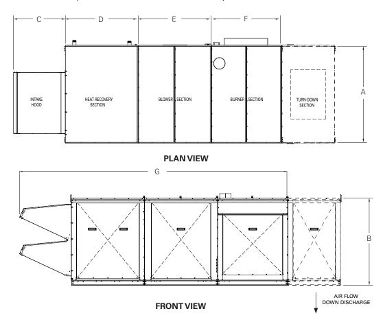
Note: Downward or horizontal discharge opening dimensions will depend on the fan type and size selected. Please refer to the job-specific submittal drawings for these dimensions.
