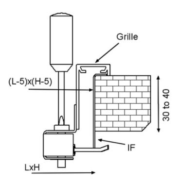
For models with a frame, concealed screw fastening is possible when the grille is installed with an installation frame (IF).
