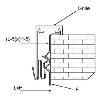
For models with a frame, the grilles are supplied with a clips fastening as standard. Clips fastening is used with an installation frame.
