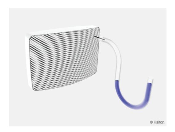
Set a probe inside the valve and measure the differential pressure with a manometer. The location for the probe would be about 20 mm from top and side surfaces.
