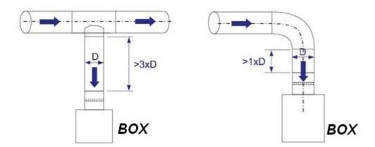
For the supply, in static pressure control, the minimum safety distance for the static measurement unit after the control damper is 5 x D in supply air applications. However, the pressure sensor position is typically halfway along or in the last third of in the last third of the duct branch length.
