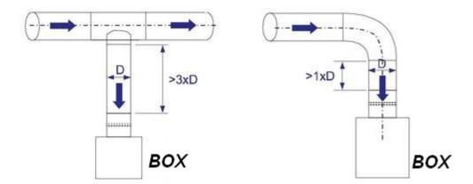
For the supply, in static pressure control, the minimum safety distance for the static measurement unit after the control damper is  $5 \times D$  in supply air applications. However, the pressure sensor position is typically halfway along or in the last third of in the last third of the duct branch length.
