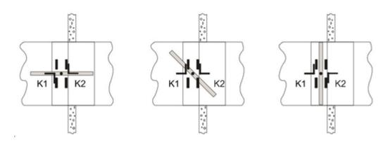
Damper open K1: 13/14 closed 21/22 open Damper drives K1: 13/14 open 21/22 closed Damper closed K1: 13/14 open 21/22 closed
