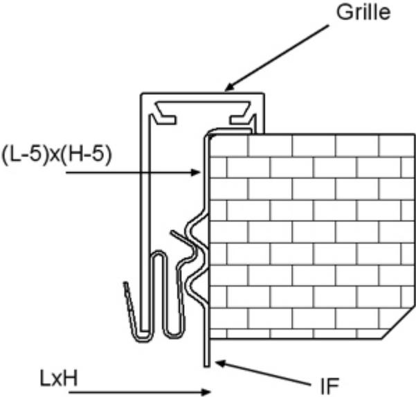
The grilles are supplied with clips fastening as standard with the IF/FLE installation frame.
