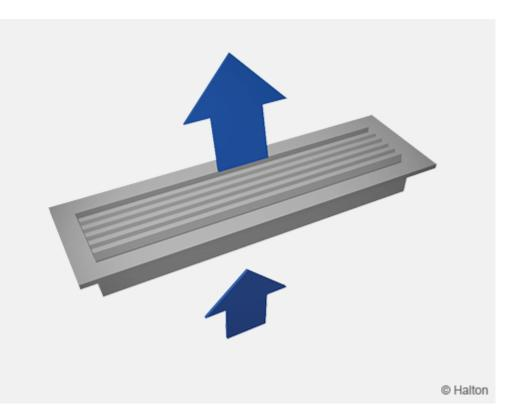
Supply air is supplied with a 15° angle deflection through the horisontal vanes into the space. Supply air mixes with room air in front of the grille. The air jet can be directed towards the wall to obtain a longer throw length.
