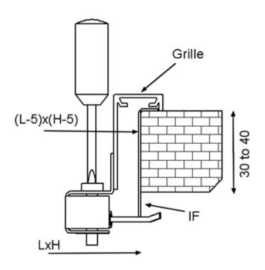
Concealed screw fastening is possible when the grille is installed with an installation frame (IF/FLE).
