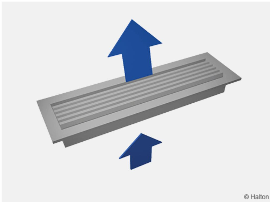
Supply air is supplied with a 15° angle deflection through the horizontal vanes into the space. Supply air mixes with room air in front of the grille. The air jet can be directed towards the wall to obtain a longer throw length.
