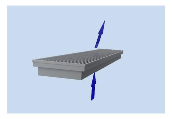
Supply air is supplied with a 15° deflection angle through the horizontal vanes into the space, and it mixes with room air in front of the grille.
