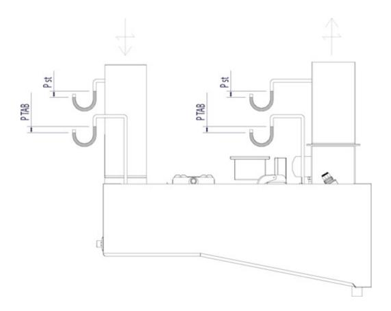
$\Omega P_{st}$  = Static pressure loss
