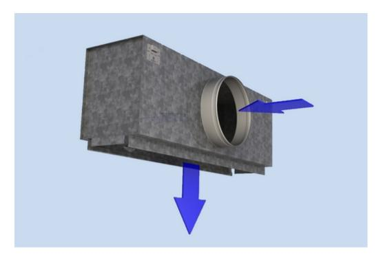
The duct pressure and air velocity are reduced inside the Halton PLL plenum box. Air is supplied into the space through the diffuser, improving the air distribution quality. The airflow rate can be adjusted using the optional measurement and adjustment module MSM.
