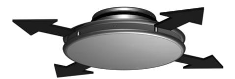
Air is supplied horizontally into the space through the side slots of the diffuser and induces the room air outside the diffuser. The recommended maximum air temperature difference between supply and room air is  $10\,^{\circ}\text{C}$  degrees.
