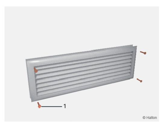
Halton TVC transfer grilles are screwed (1) either to the wall or door, on both sides (2 x TVC, if required).
