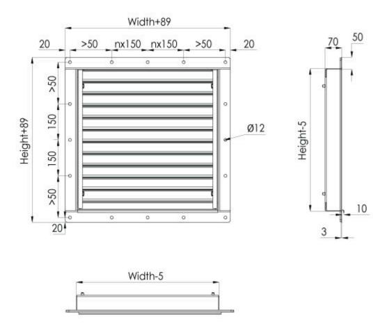
The USM louvres are manufactured for rectangular openings with widths (B) ranging from 150 to 1500 mm and heights (H) from 150 to 2400 mm, with a 1 mm division. Modular construction is available for larger sizes. Special flange configurations are available on request.
