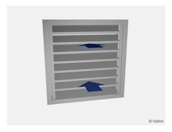
Air is supplied or extracted through the horisontal blades. The design of the grille prevents rainwater from reaching the ductwork. The slot between the frame and the top blade is sealed, thus preventing rainwater from entering the ductwork from above. Drops of water are collected in the grooves at the front edge of the blades. Water flows to the side grooves, where it drops down.
