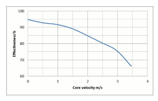
Water penetration rating per square meter of louvre tested according standard EN 13030:2001. Core velocity at free duct area of louvre size.
