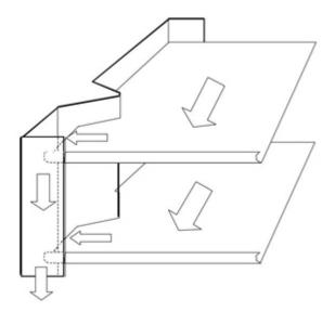
Depth of blade 65 mm, distance between blades 50 mm, free area 50%
