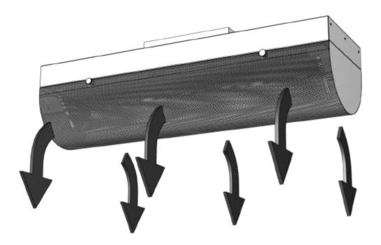
Supply air is supplied with low-velocity from the galley ceiling. The air flows into the galley without causing a high velocity draught and turbulance that could effect on hood extraction efficiency.
