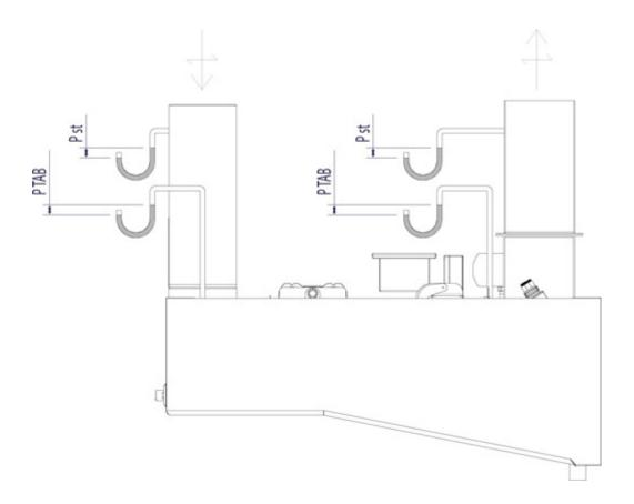
$\Omega P_{st}$  = Static pressure loss
