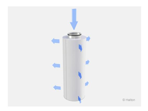
Air is supplied into the space uniformly through the front panel of the unit, generally at a slightly lower temperature than the room air. The supply air flows down to the floor level, before gradually pervading the occupied zone at a low velocity. Finally the convection of warm surfaces causes the air to rise out of the occupied zone. The low velocity flow pattern is circular (360°). The low velocity flow pattern is directed forward.
