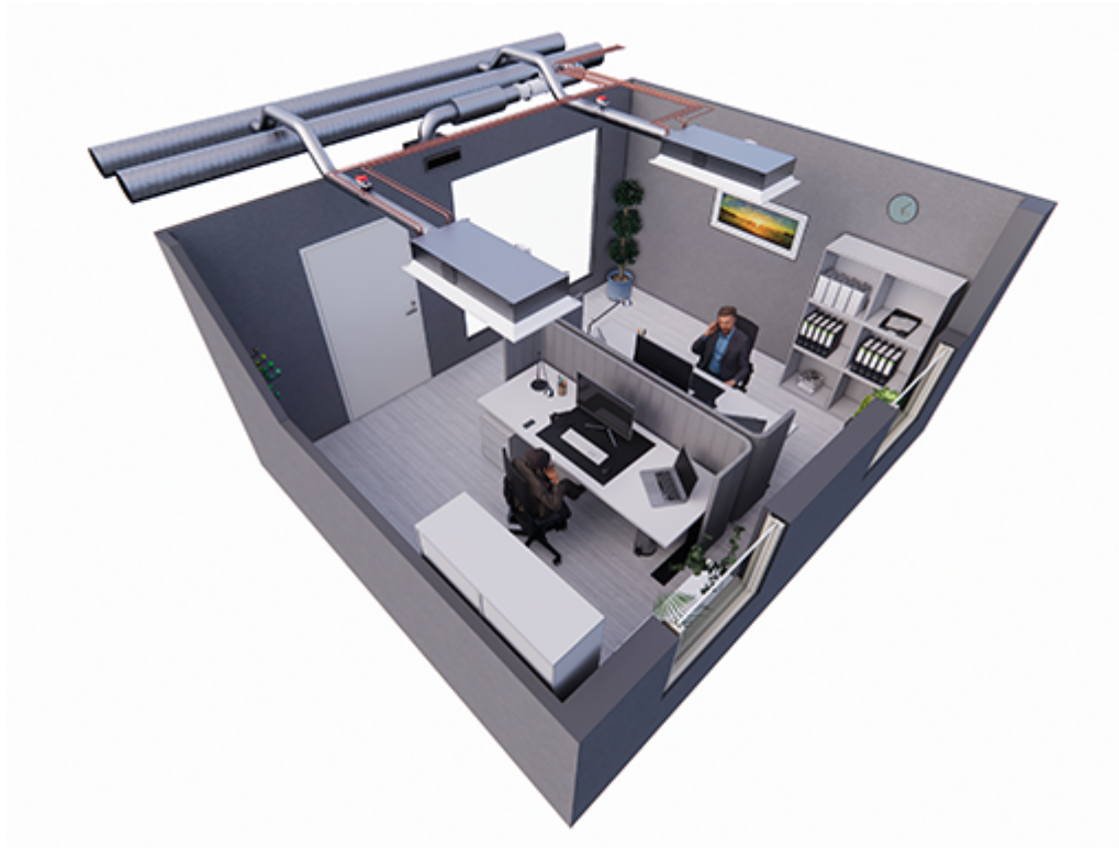
Fig. 11. Halton Rex RXP active chilled beams with HAQ control and PTS damper, controlled with Halton Workplace WRA room automation controllers in a double office room
