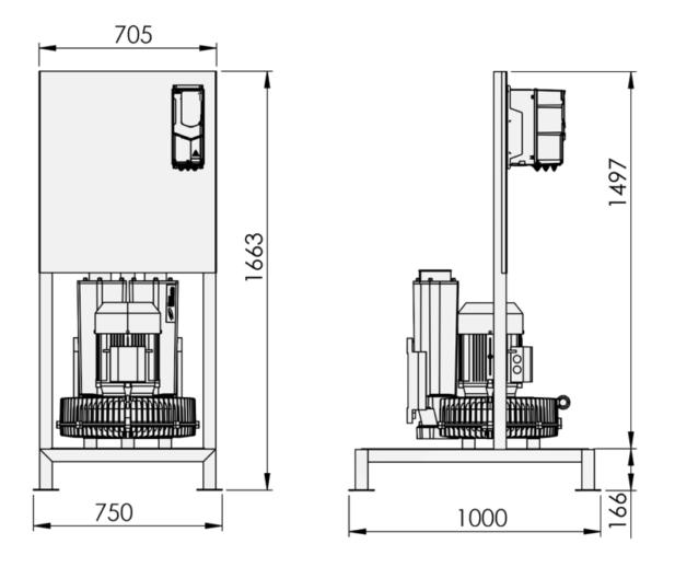
Fig.4. Dimensions of Halton Vita Extract central unit (single)
