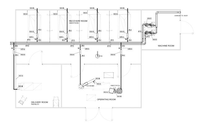
Fig.3. Plan drawing example of a Halton Vita Extract system
