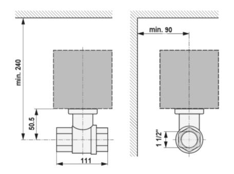
Fig.7. Control valve dimensions
