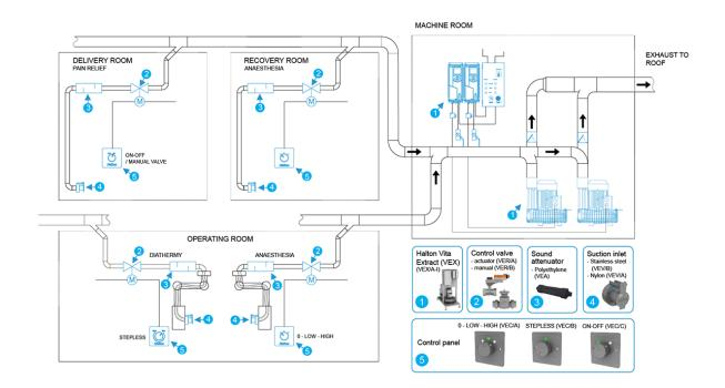
Fig.2. Overview of Halton Vita Extract system components
