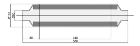
Fig.8. Sound attenuator dimensions
