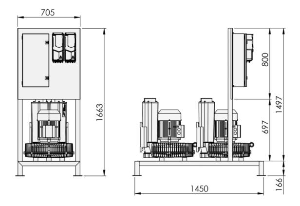
Fig.5. Dimensions of Halton Vita Extract central unit (dual and secure)
