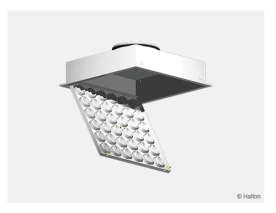
Detach the front panel of the diffuser by gently pulling it down and let it balance on the hinges. Each nozzle can be easily removed by pressing the stoppers and then pushing the nozzle through the front panel.
